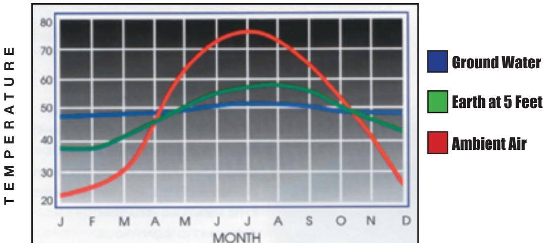
*The year 'round stable temperatures of ground water and the earth itself make it possible for the energy exchange to occur in geothermal systems.*
